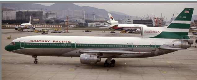
CX Tristar... Note the MAS DC-10 in the background with clearly different number 2 engine
